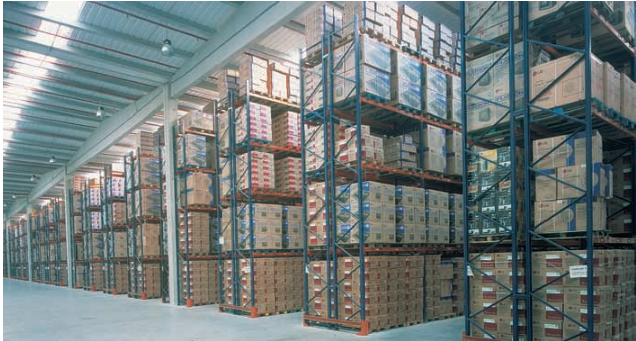
Conventional pallet racking warehouse. Pallet handled by side measuring 800 mm.
