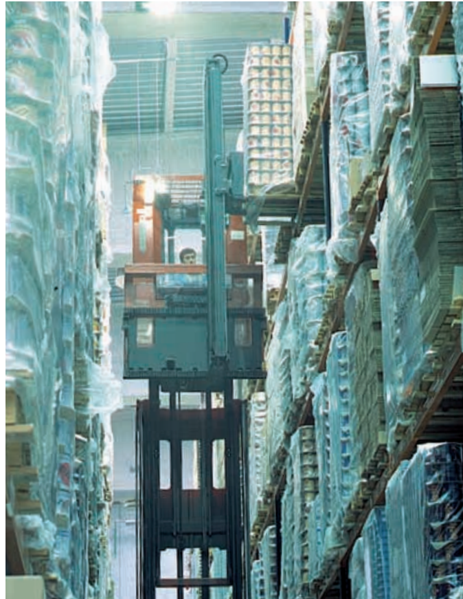
Three-position forks in insertion/extraction position.
