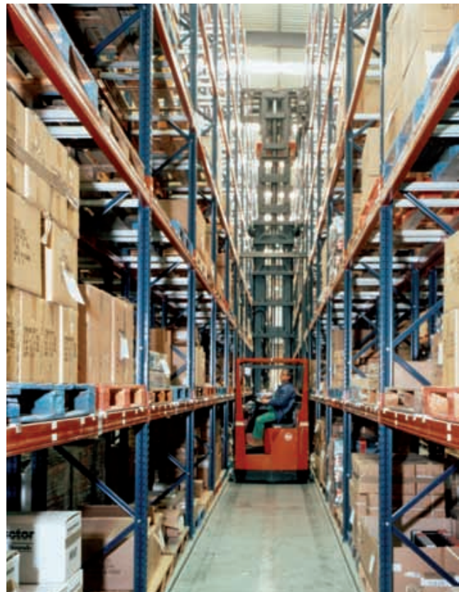
Pallet racking system with 7 load levels. Pallet handled by side measuring 1,200 mm.
