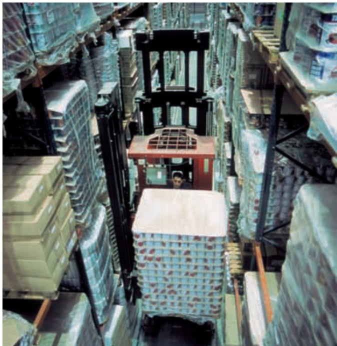
Three-position fork in circulation position.
